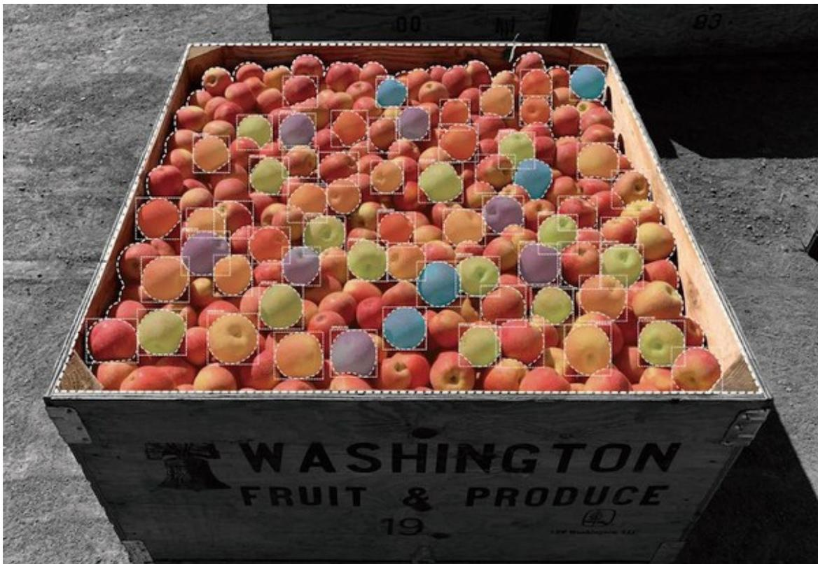
*Inside the tech: Using computer-vision technology, Spectre begins detecting apples in the bin and delivers sizing results within seconds.*
