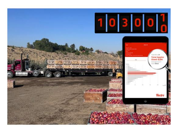
Spectre Top Down is Hectre's overhead early fruit sizing AI solution. A camera installation is connected to Hectre's computer vision sizing app, Spectre. Trucks arriving at the receiving site simply pass under the camera and their load is scanned.
